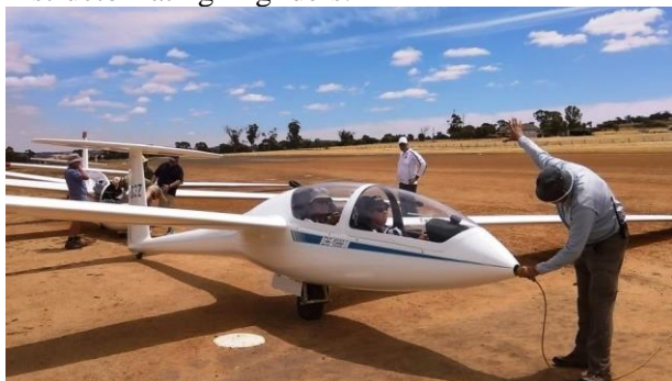
Davis Walmsley getting his tow cable release mechanism checked prior to gliding at Beverley
